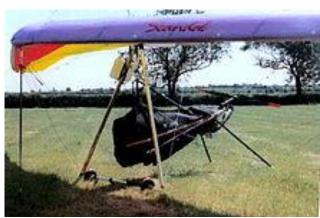
The Mosquito Powered Harness for a foot launched powered hang glider designed and produced by Swedish inventor Johan Åhling, of Swedish AeroSport.
